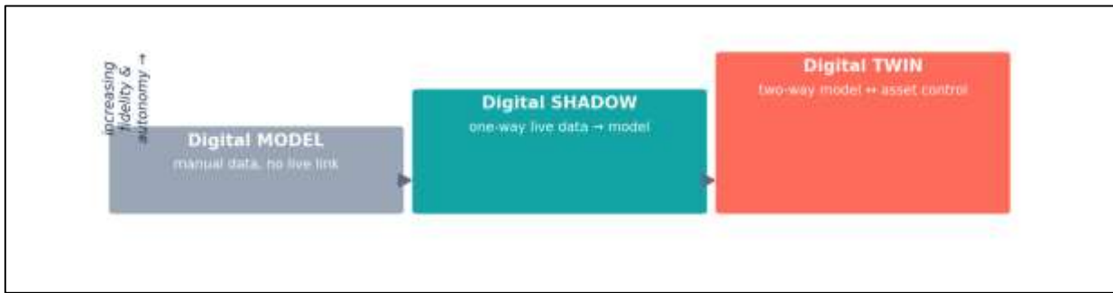
Figure 3: Digital Twin Maturity and Data-Synchronization Workflow
